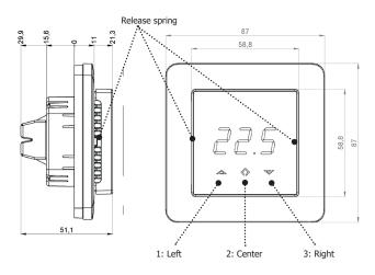
Use e.g. a small slotted screwdriver. Start by carefully removing the front cover by pushing the release springs. The front cover and the frame can now be removed.
