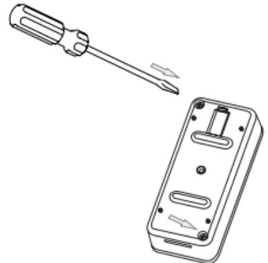
2. Separate the battery cover from the Sensor unit.
