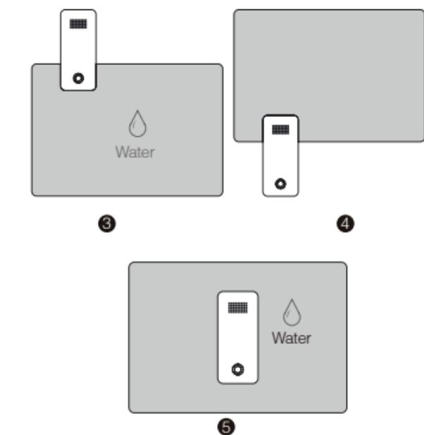
The above situations are the water leak or water presence event is triggered by the Sensor, when the water recedes from the Sensor, the water leak event will be cleared and then the Sensor will
