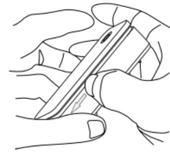
3. Battery cover is separated from the Sensor unit.
