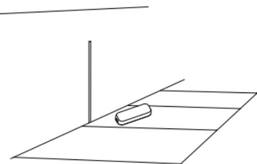
If you want to detect whether or not there would be water leakage from the fridge, you can put the Water Sensor near to the fridge. Just note that the Water Sensor cannot be put inside the fridge or other metal container, since the metal container
