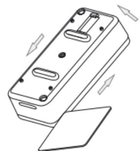
You can also open the battery cover through your fingers if you are confident about this way. Find the position of the screw side, see the operating steps below:
