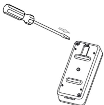
After complete the securing of the Sensor plate, your Water Sensor unit will possess the high waterproof level of IP65.
