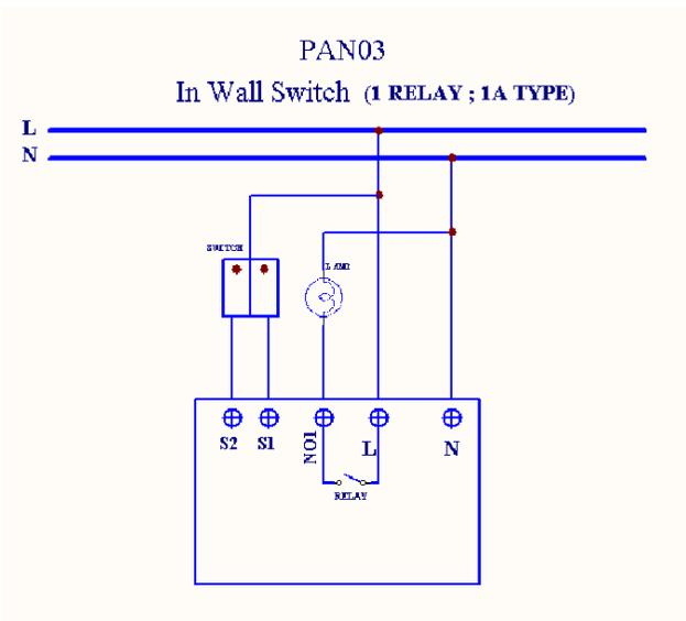
**Fig 1. PAN03 Assembling**
