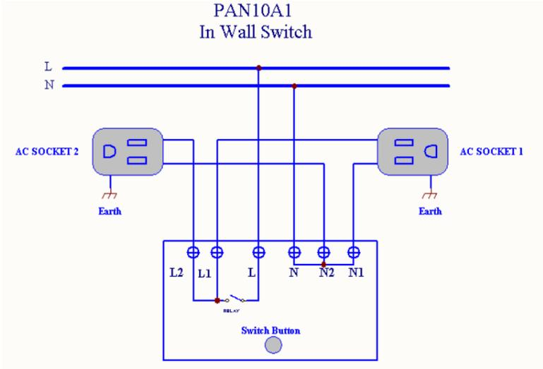
**Fig 2. PAN10 Assembling**
