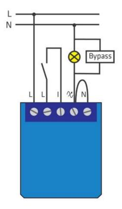
(i) NOTE: When installing the Mini Dimmer in a 2-wired installation, if the load connected to the output starts flickering, we recommend you use a Bypass. Bypass is designed to be used with LED loads.
