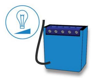
The Qubino Mini Dimmer is 25% smaller than any other wireless dimmer in the world. Mini Dimmer is a MOSFET-switching light device that also supports control of low-voltage halogen lamps with electronic transformers, dimmable compact fluorescent lights, and dimmable LED bulbs. It can work with or without the neutral line (3 or 2-wire installation).
